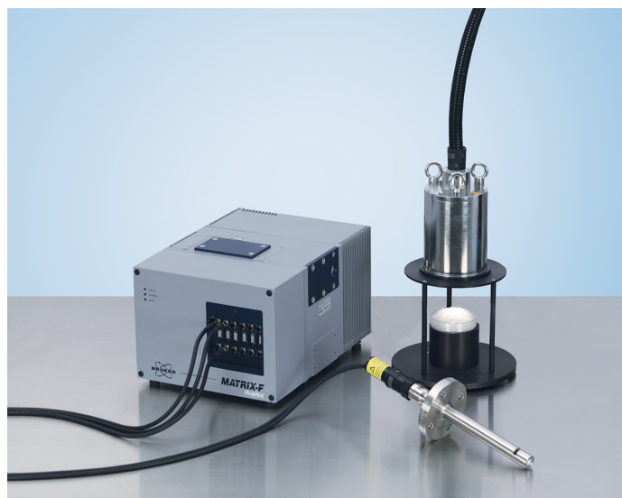
Bruker Matrix-F with a transmission probe mounted on channel1 and a contactless reflection probe connected to channel2. The system can be equipped with up to six completely different probes for monitoring up to six independent sampling points/reactors.
